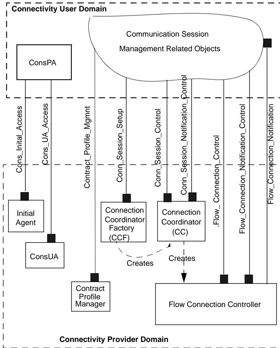
Figure 4-1. Cons-RP Computational Architecture
